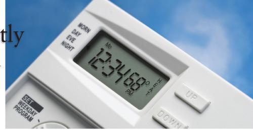
are absent or asleep. Programmable thermostats can be retrofitted, so it's possible to keep the same furnace and replace the thermostat.
